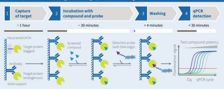
The target is captured to a solid phase via appropriate anchor and incubated with screened compounds together with the DIANA probe made of small-molecule inhibitor attached to a reporter DNA. The inhibition potency is directly determined using quantitative PCR. DNA-linked substrates or ligands can also be used as probes.
